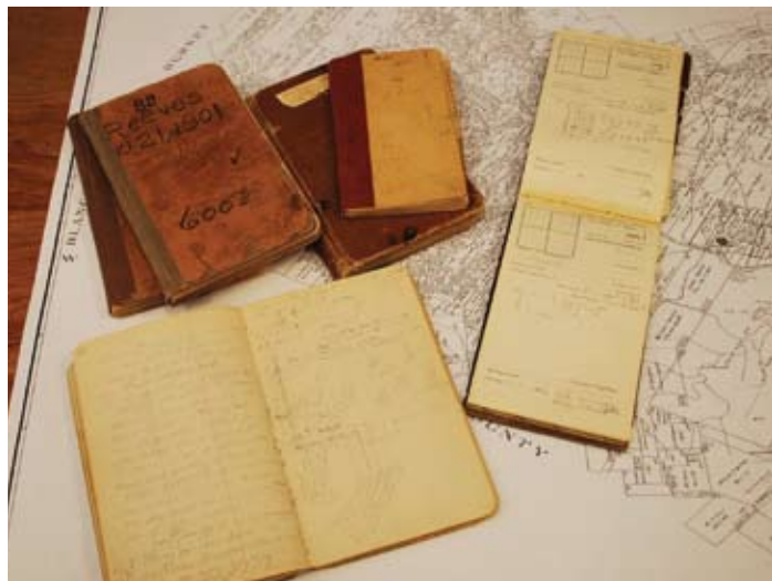
Examples of field books found in the Twichell Survey Records. Field books—the notebooks that surveyors make on the ground—are particularly valuable as they contain sketches, computations, and notes from which official field notes and maps are created.
