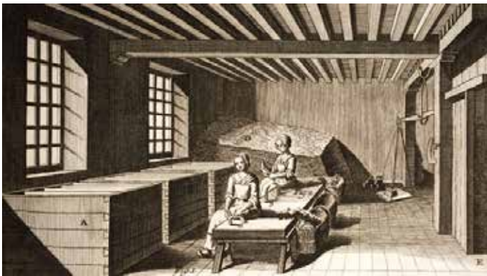
This illustration from Diderot's Encyclopédie shows women sorting rags. A carefully sorted batch with similar weight, color and so-called tenderness ensured predictable results during subsequent operations.
